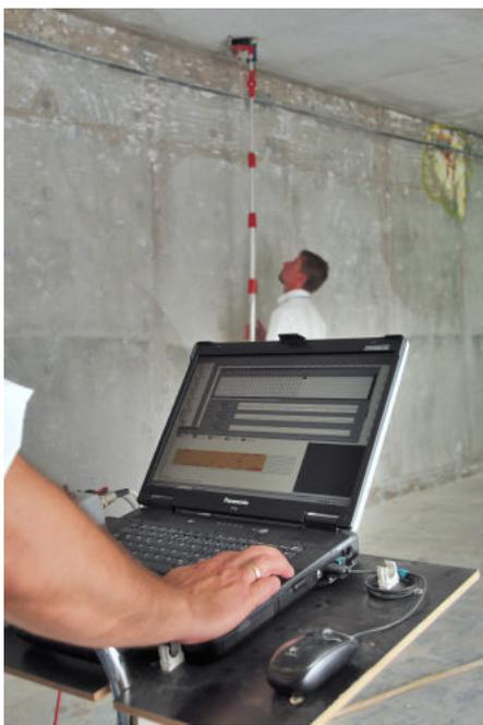
Fig. 3: Recording potentials and resistivity.
