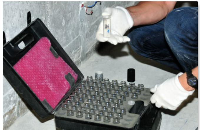
Fig. 5: Collecting drill dust samples.
