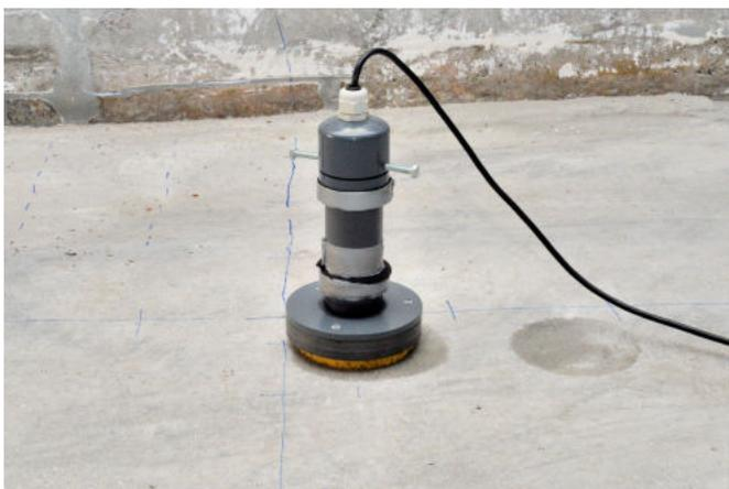
Fig. 10: KMS-probe0 (System CiTec) for LPR-, Galvanostatic Pulse- and Tafel-tests.
