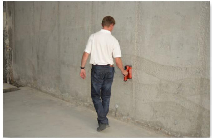
Fig. 4: Measuring concrete cover.
