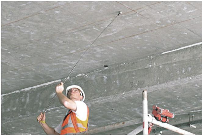
Fig. 2: Delamination check.
