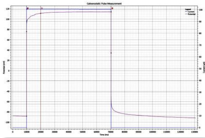
Fig. 8: Galvanostatic pulse measurement.
