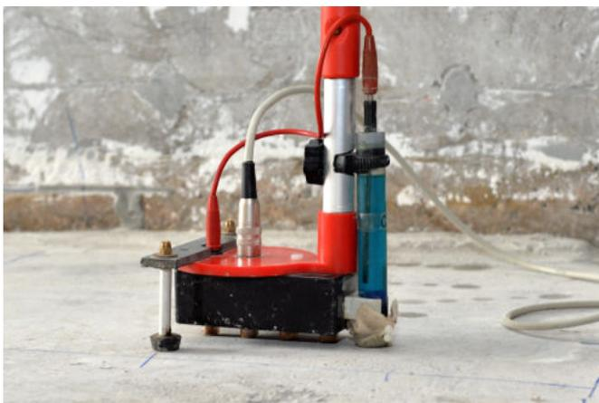
Fig. 7: Combination probe for potential and resistivity measurement (System CITEC).
