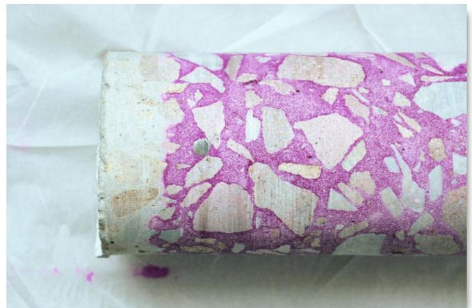
Fig. 6: Checking carbonation depth on a core sample using an indicator liquid.
